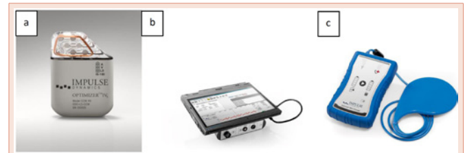
Figure 2 : a) Optimizer IVs Active Implantable Pulse Generator. b) Device programmer. c) External charger used to recharge the battery of the generator on a weekly basis.
