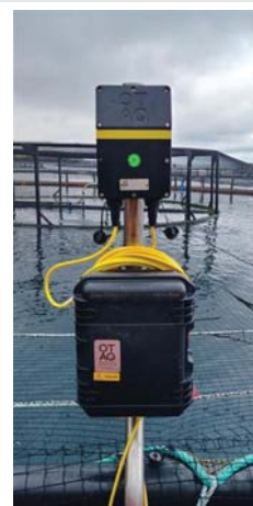
Figure 2: Single R&D patrol mode OTAQ Aquaculture SealFence AHD unit on Isle of Skye fish farm, Scotland. 16 units were present on the farm.
