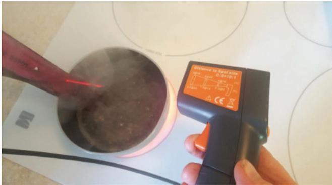
**Figure 7a:** Apparatus for measuring the temperature of steam as a function of height above a boiling water surface. Temperatures were measured with an infrared thermometer. The light ray from the device, invisible in air, is visible in the steam cloud, much like in a cloud chamber. The ray reflects off a plastic ruler which formed a temperature gradient above the water.
