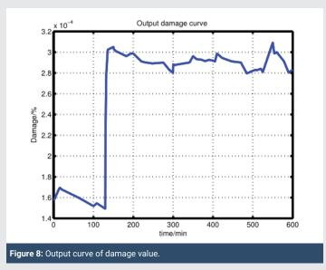
As can be seen in the figure, after the start of the impulse process, a large number of high temperature and high pressure steam enters the cylinder, and the heat is continuously released on the rotor surface, resulting in the increasing thermal stress of the rotor, so the real-time data of low cycle fatigue damage is maintained in a high level data fluctuation.
