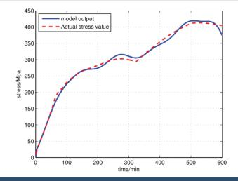
Figure 7: Comparison of actual stress and model output stress.
