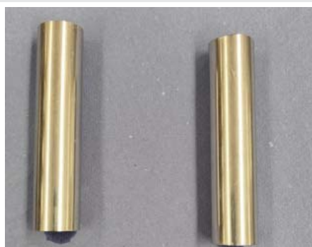
Figure 11: Specimens after contact 1 hour at 175 °C in oil.
