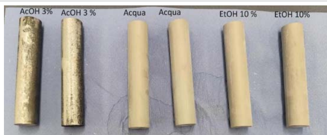
Figure 9: Specimens after contact 10 days 60 °C in Acetic acid 3%, Water, Ethanol 10%.
