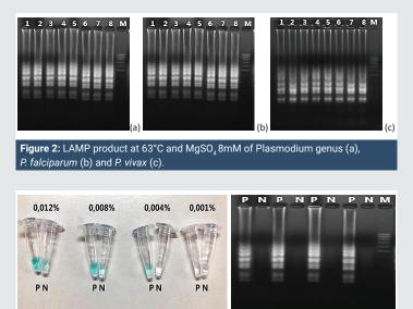
Figure 3: MG concentration tests at 0.012%, 0.008%, 0.004% and 0.001% at 63°C for 60 min. P lane and N lane represent positive and negative reactions, respectively.
