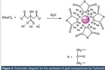
Figure 2: Schematic diagram for the synthesis of gold nanoparticles by Turkevich method.
