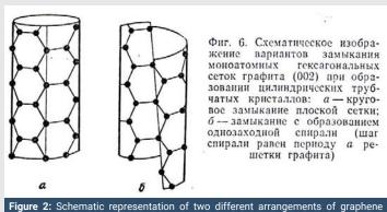
hexagonal nets (002) rolled into a cylinder, published in [4]: (a) armchair tube, (b) chiral tube (the helix pitch is equal to the corresponding lattice parameter of graphite).
