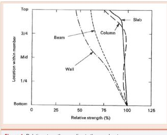
Figure 1: Relative strength according to the member type.
