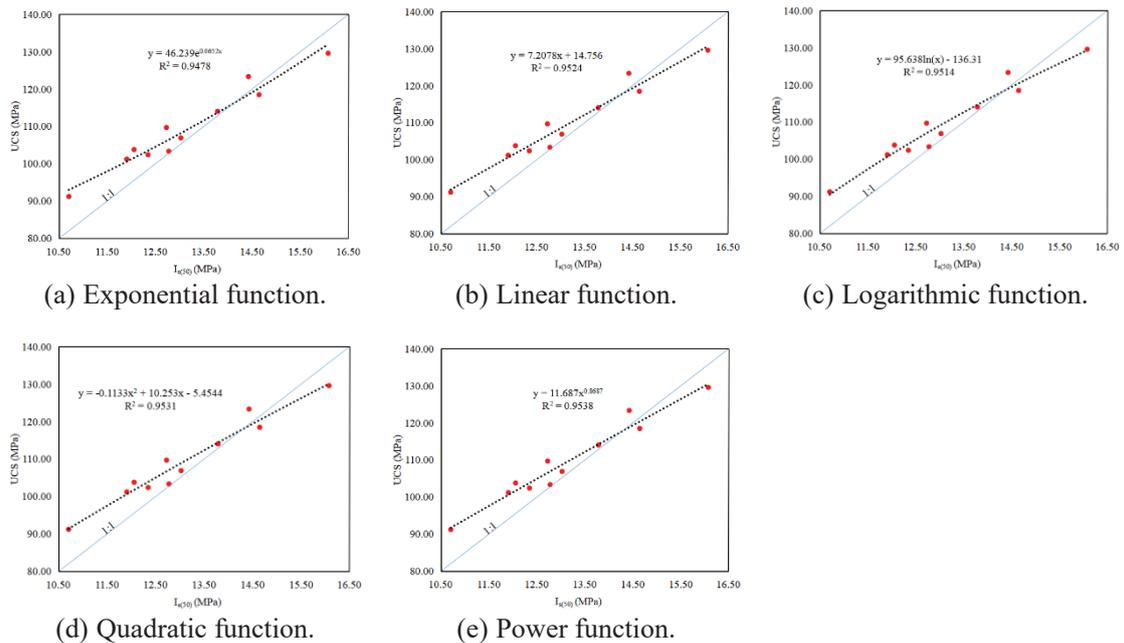
Figure 7: The functional relationship of  $I_{s(50)}$  and UCS for vertical stratification.
