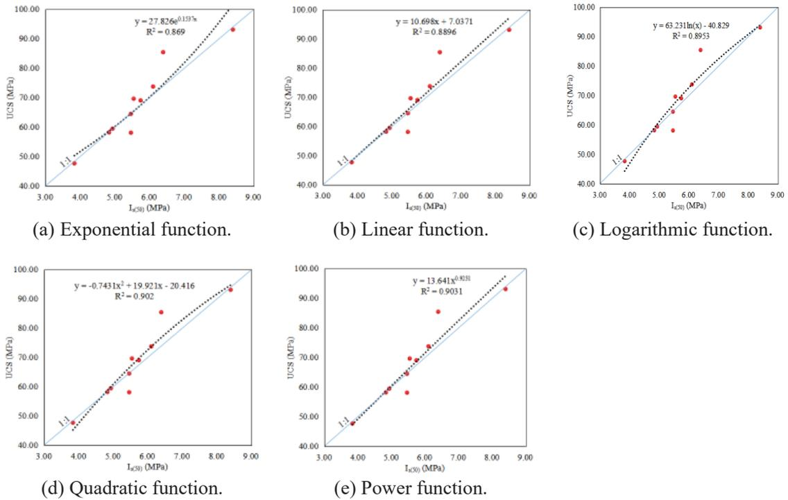
Figure 6: The functional relationship of  $I_{s(50)}$  and UCS for parallel stratification.
