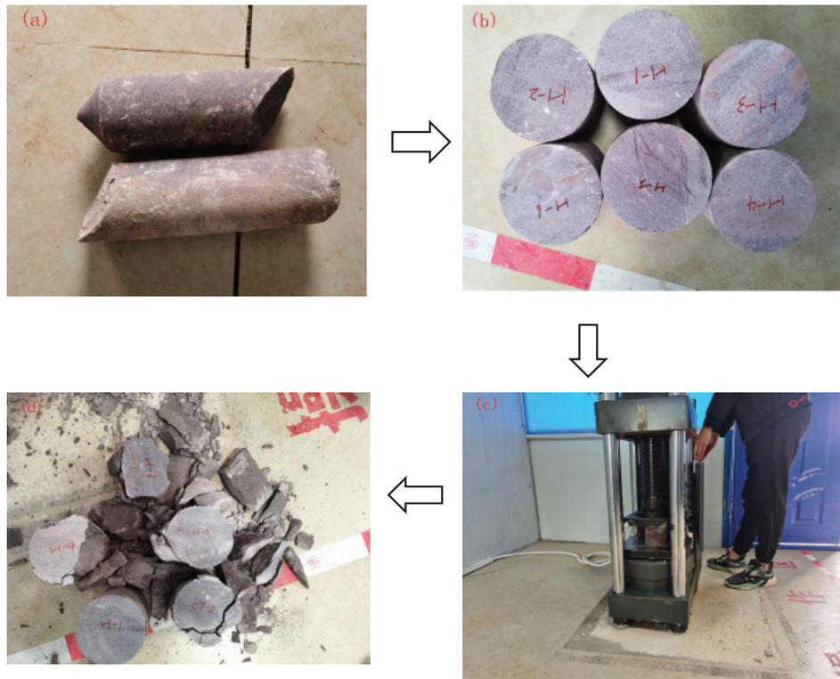
**Figure 2:** Test process of rock samples. (a) The rock core samples were taken from the field, (b) The processed rock core sample, (c) Test process of UCS, and (d) The rock core samples after the test.
