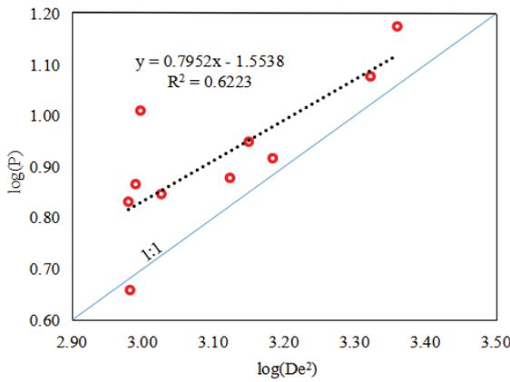
Figure 4: The logP-logD<sup>2</sup>e curves of parallel stratification.
