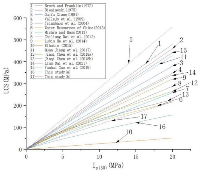
**Figure 8:** The comparison of the conversion relationship between  $I_{s(50)}$  and UCS from different researchers.
