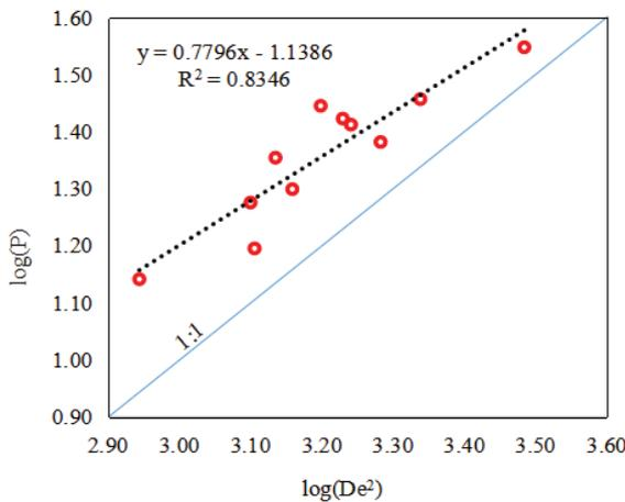
Figure 5: The logP-logD<sup>2</sup>e curves of vertical stratification.
