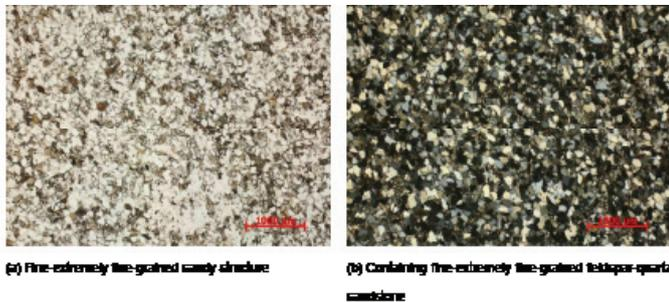
Figure 1: Microscopic analysis of the sample under a microscope.
