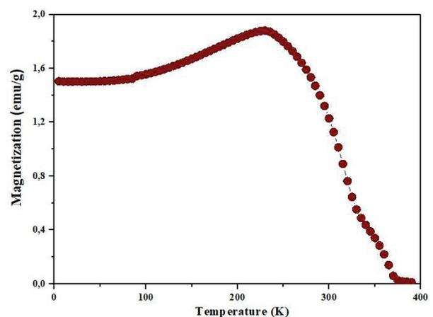
Figure 3: Variation of the magnetization as a function of temperature for  $\text{Sr}_{0.6}\text{Ag}_{0.4}\text{MnO}_3$  nanoparticle.
