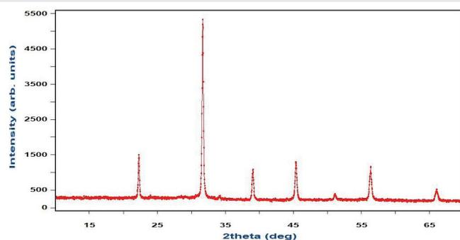
Figure 1: Powder XRD patterns of  $\text{Sr}_{0.6}\text{Ag}_{0.4}\text{MnO}_3$  nanoparticle.
