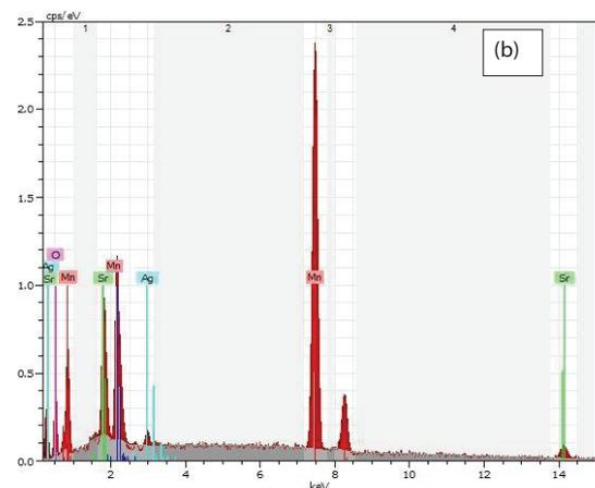
Figure 2: Image SEM (a) and EDX spectra (b) of  $\text{Sr}_{0.6}\text{Ag}_{0.4}\text{MnO}_3$  nanoparticle at room temperature.
