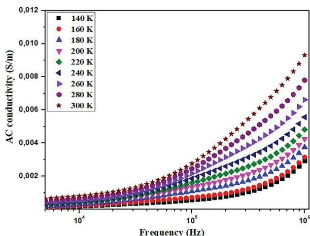
Figure 4: Variation of AC conductivity with frequency.
