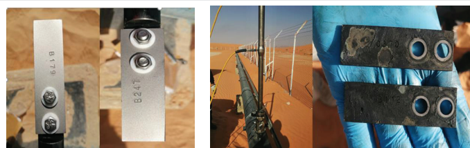
Figure 6: Corrosion coupons before installation and after extraction on the 8-inch (8") line – 45 Day exposure period.
